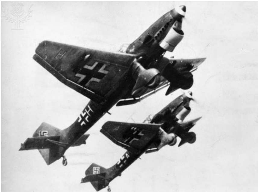
Figure 3: Two Stukas equipped with their iconic air sirens. The sirens were mounted on the gear legs just below the wings. German bombers – German Stuka dive bombers photographed, c1942, during World War II. Encyclopedia Britannica ImageQuest, photograph.
