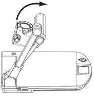
4. Move the lamp column and the lamp head to an appropriate position.
